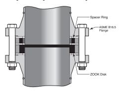
When replacing a metal rupture disk with a ZOOK Graphite Rupture Disk, a graphite lined armored spacer ring can be provided to fill the space of existing flange face-to-face distance, eliminating the need for piping modifications.
